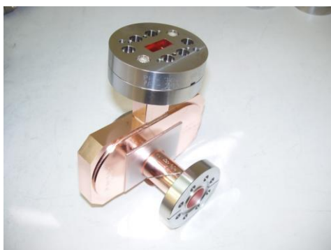
Figure 8. Mode launcher to be prepared for the KEK basic study setup.
